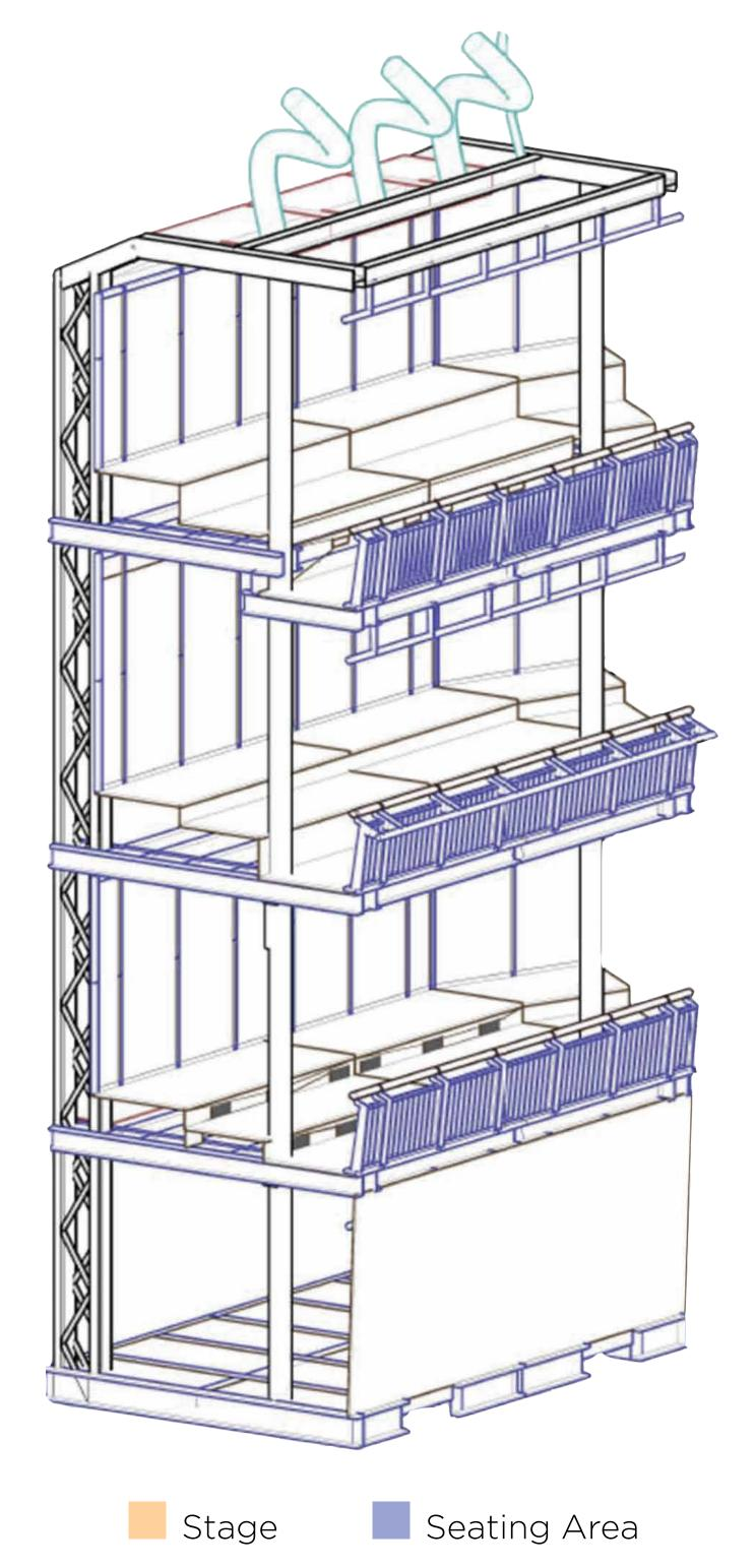
Each mobile tower—the size of a city bus stood on its end—contains three levels of seating. These complex structures, pioneered for this design, house extensive theatrical technology, and connect into a network of HVAC components and sprinkler systems to accommodate audience comfort and safety.
